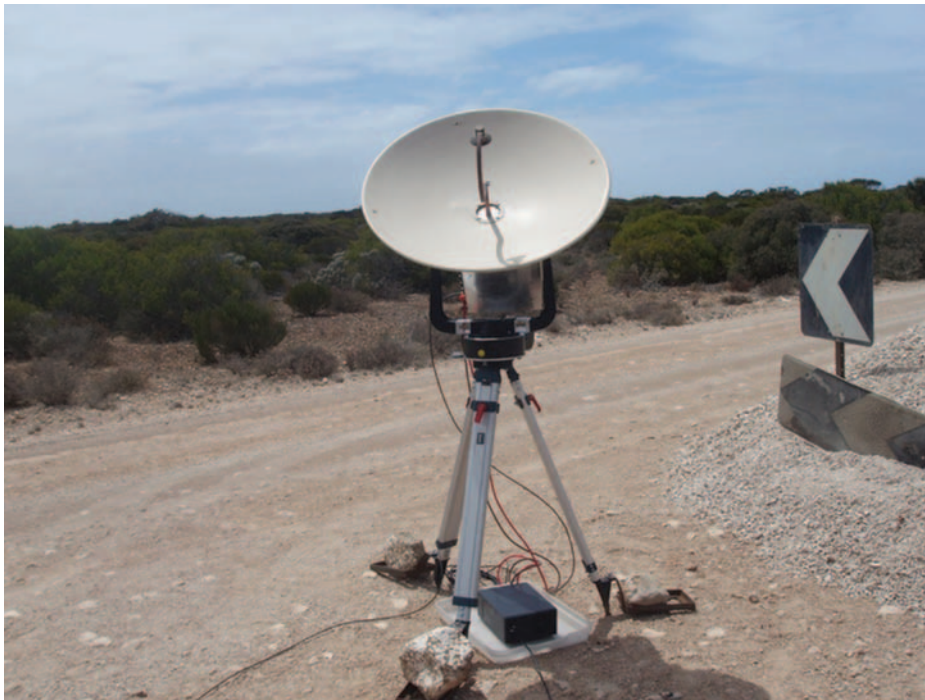
PHOTO 2: The portable EME-capable 10GHz station of VK7MO, set up at a roadside in the Australian outback.
