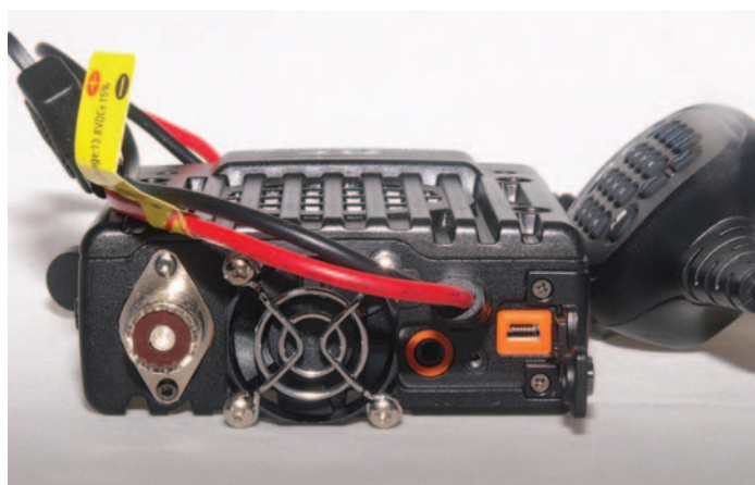
The rear of the TYT TH-8600 showing the USB data connection (orange).
