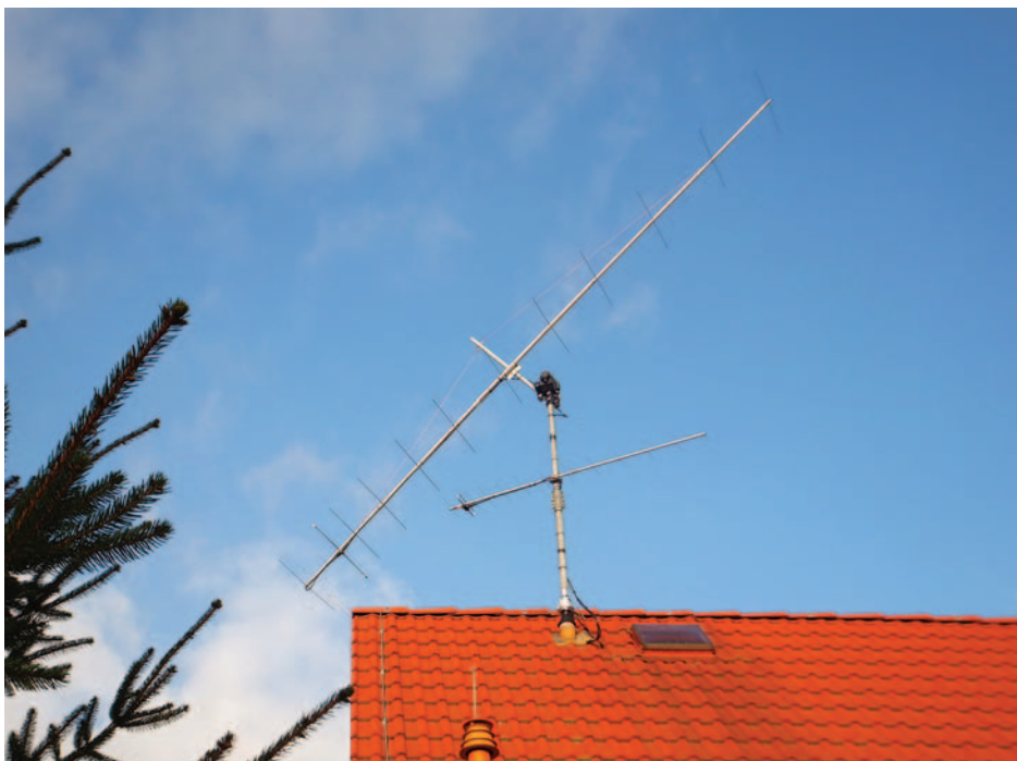
PHOTO 1: The 12-element Yagi antenna used by DL1VPL to complete DXCC on 144MHz.
