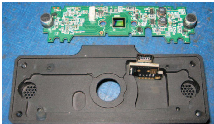
PHOTO 7: Main board and aluminium case front with new USB socket and carrier board in place.
